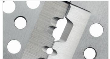
Two pairs of blades (1) cut the insulation to a complete extent. Then the blade pairs move apart, and thus the insulation is removed form-fit (2). The pliers opens automatically after the stripping procedure.
